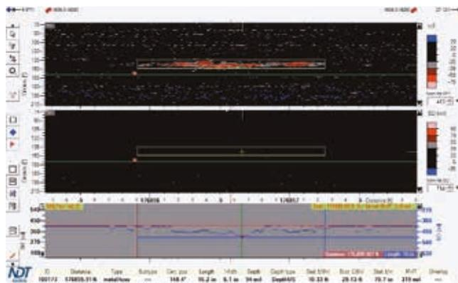
Figure 5. C-Scan representation of wall thickness data. Top: wall thickness reading. Bottom: stand-off data.
