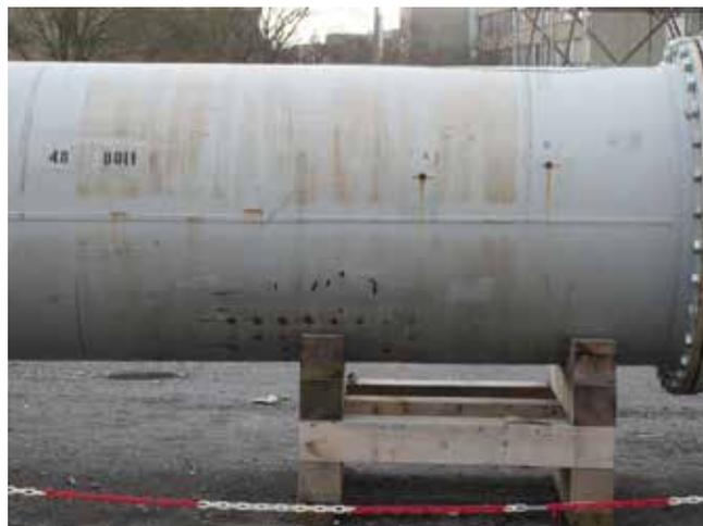
Figure 4. Photograph of 48 in. test spool with test defects.
