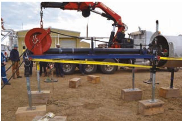
Figure 3. Picture of launching tube connected to transport frame.
