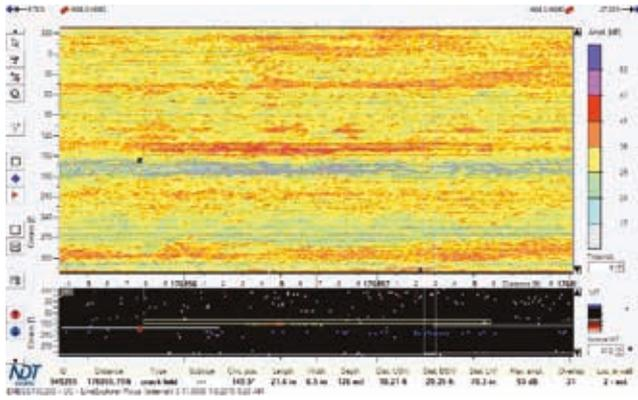
Figure 6. C-Scan representation of crack data. The red box indicates a crack-like anomaly defined by the automatic boxing algorithm.
