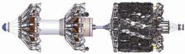
Figure 1. Design of two segment 36/48 in. multi-diameter UM/UC combo tool. The pull unit with batteries (left) and sensor carrier with tool electronics (right).
