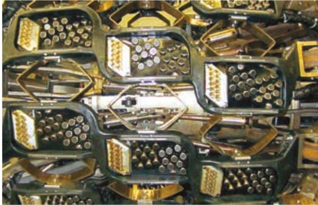
Figure 2. Photograph of the expanded sensor carrier mounted on transport frame. Three groups with black/grey (crack transducers) and silver/bright (wall thickness transducers) are visible within each skid.
