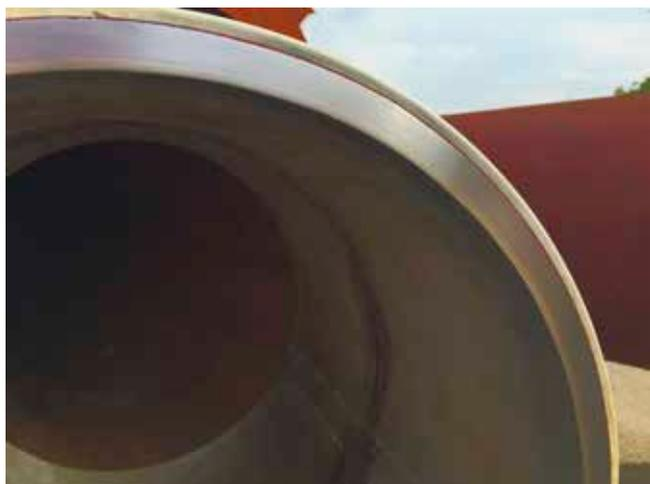
Figure 1. Cross section of a CRA lined pipe.
