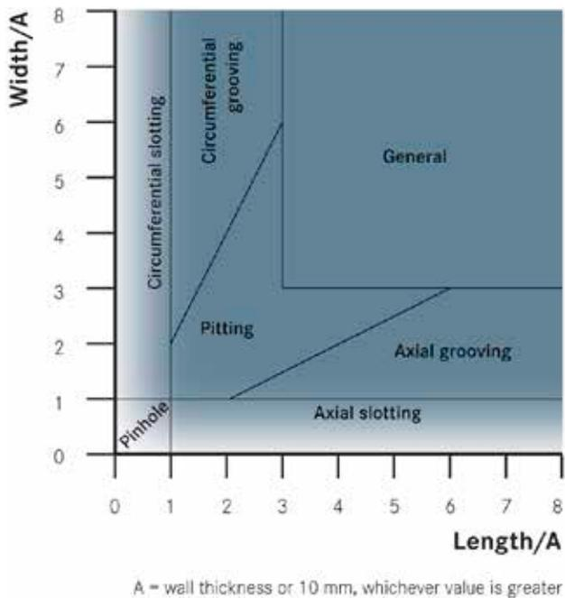
Figure 3. Metal loss feature classification according to POF and API 1163.
