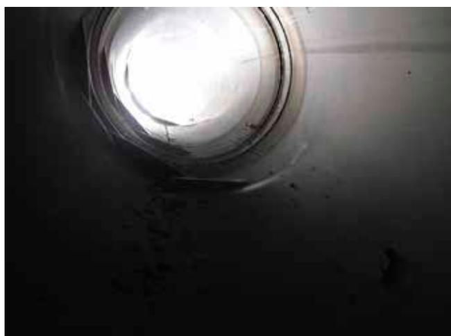
Figure 2. Example of wrinkling and buckling in a CRA lined pipe.
