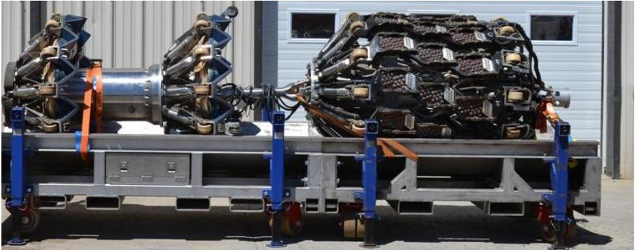
Figure 8: 36/48" UT crack and wall thickness combo tool
