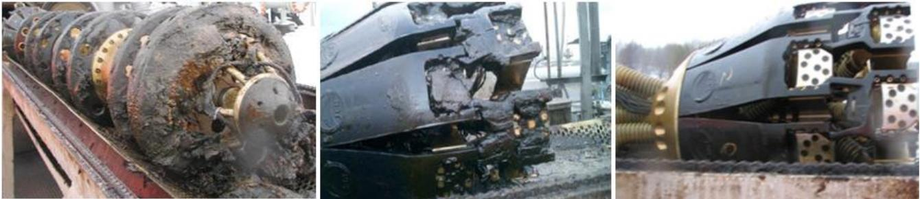
Figure 4: Left and center: conventional UT tool after inspection of wax rich pipeline; right: sensor carrier with flushing system after inspection of identical pipeline.
